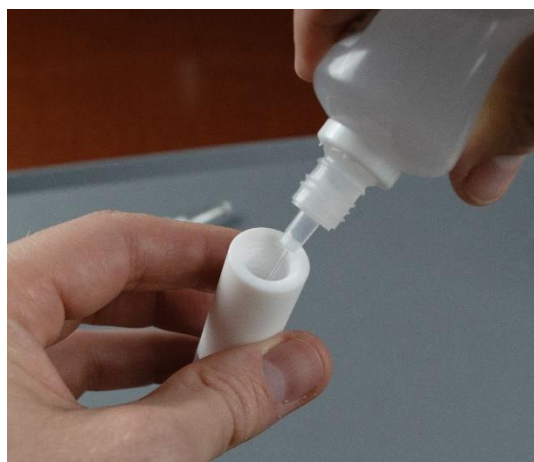
Image 11. Filling up the Electrode Chamber in Step 14.
