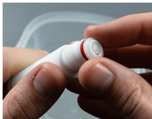
Image 3. Placing an Electrode Membrane on top of the Cathode Plate
