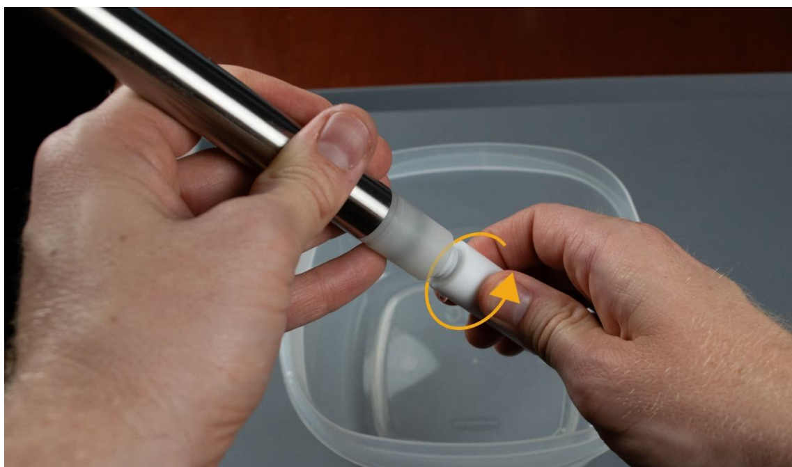
Image 12. Screw the ECEG fully onto the Electrode Body.
