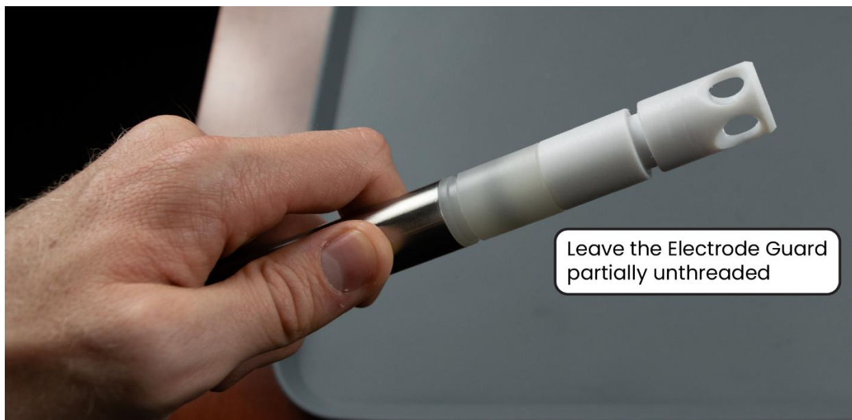
Image 5. How the sensor should look after Step 5
