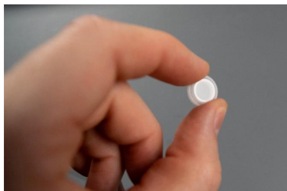
Image 2. Safely holding an Electrode Membrane
