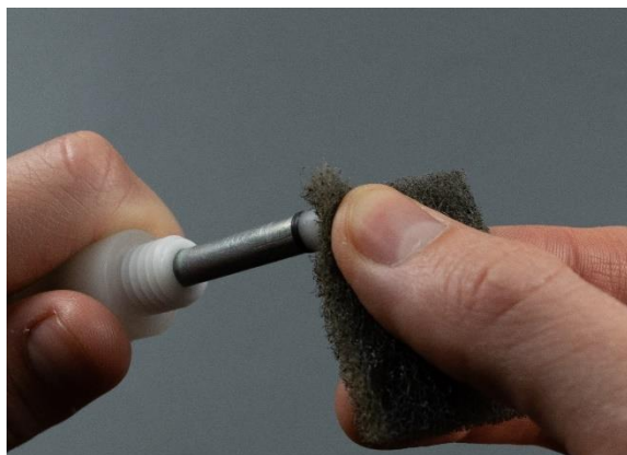
Image 9. Rub the Scouring Pad across the Cathode Plate.
