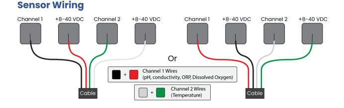
D-phi Series<sup>™</sup> sensors have Reversible Input Protection (RIP). This means that the red and black wires function interchangeably as the power and output. RIP prevents damage occurring to the receiver or sensor due to improper wiring and simplifies the wiring process.
