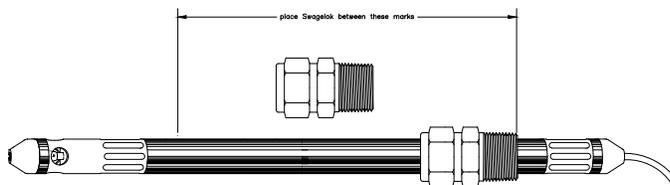
For most parameters (except for conductivity and temperature) the sensor end of the sensor/transmitter should be angled at least thirty degrees below the cable to prevent air entrapment in the reference solutions or measurement electrode. *Care must be taken to assure that the stainless-steel housing is contacting the solution to be measured – or the differential amplifiers will not perform properly – making the measurements appear to be erratic.*
