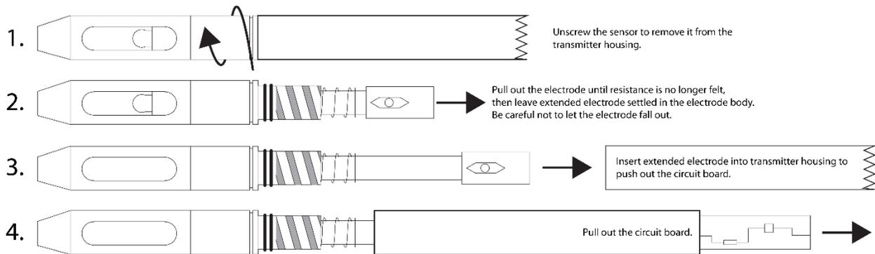
Pay attention to which end was facing the cable to allow for proper alignment when reinserted.
