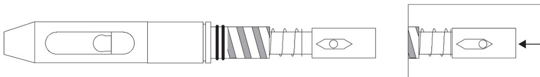
10. Reinsert electrode body into transmitter body and screw in until plastic is flush with metal body.
