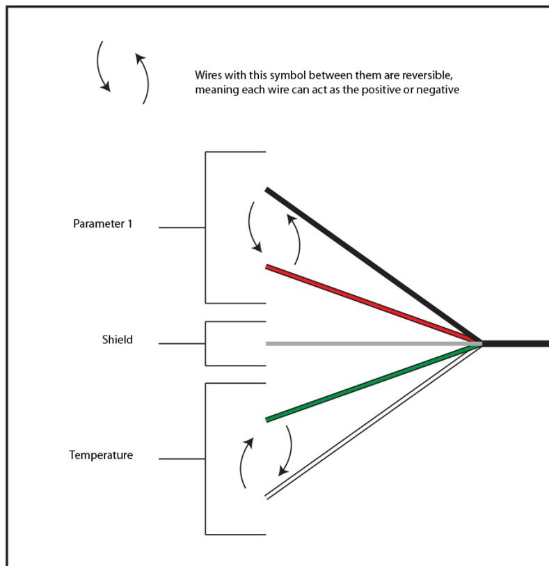
The auto-polarity correction feature directs the applied supply voltage to allow for proper operation regardless of wire hookup. The **RED** and **BLACK** wires are for channel 1 -- pH, and the **WHITE** and **GREEN** wires are for channel 2 -- temperature. The electrode can be replaced in 15 seconds -- further reducing costs.
